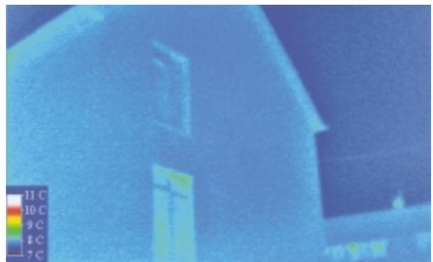
The image above shows a **Kingspan TEK® Building System** gable wall with a relatively even surface temperature. Very little thermal bridging can be identified. There is also no visible air leakage at the verge. It should be noted that the rooms behind the are well heated which further displays the well insulated nature of the construction.
